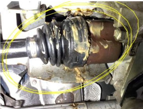
drivers side CV shaft boot leaking grease
