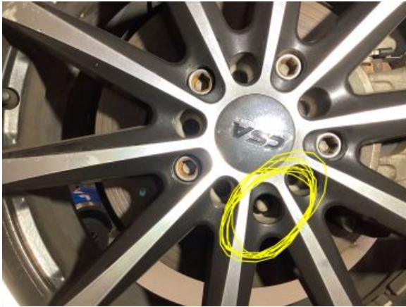
right front wheel nut missing
