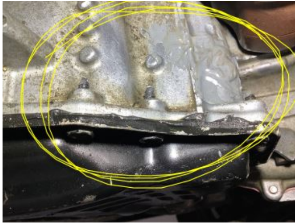
auto transmission case repaired with silicon/leaking
