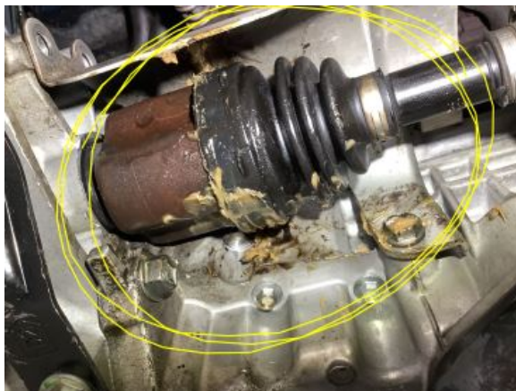
grease splashed out from Cv boot
