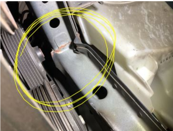
drivers side chassis bent/kinked
