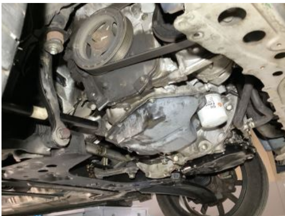
stone guards/splash tray missing underbody
